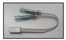
The Vegsensor is a thermal switch which operates in the temperature range of ~65C to ~90C. When installed with a VEG-Therm in line electric heater, it will only activate the heater when the temperature range is reached, eliminating the need for a separate toggle switch.
